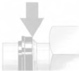
Fig. T50 — Ferrule cocked on tube
