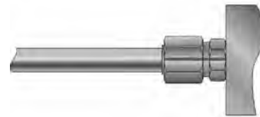
Fig. S32 – Make reference mark on nut and tube body
