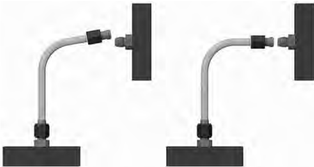
Fig. S31 – Improper bend and short tube
