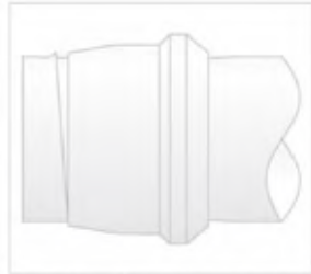
Fig. T50 — Ferrule cocked on tube
